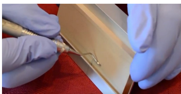
Student 3rd technique: Fulcrum on table move entire fixture/stone
